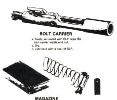
a. Wipe down inside, outside of the tube, the spring
